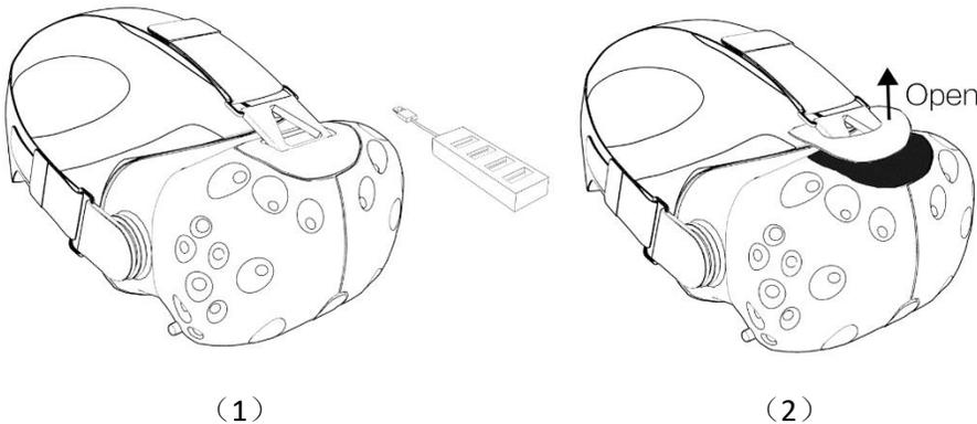
2. Plug the 1-to-4 USB Hub into any free USB slot on the Headset.
