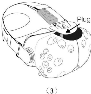
3. Re-install the USB slot cover, fix the 1-to-4 USB Hub on Headset using the elastic band, plug in two Dongles and have fun.
